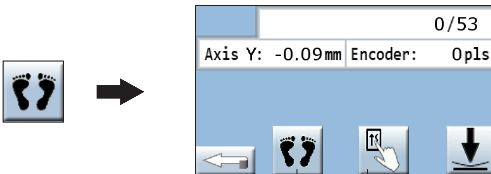
① Activation of tack step-by-step sewing mode ② Proceed to next stitch
