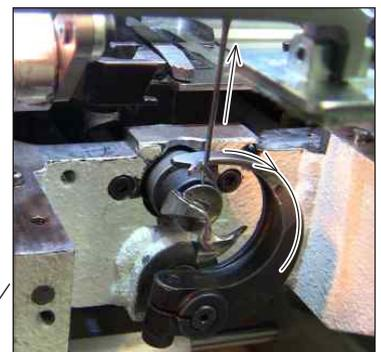
The setting shall be performed by the screw of the smaller eccentric – refer to the picture below.
