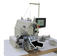
**2. Horizontal button feeder position:** insert the button gauge
