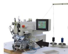
The needle shall be in one line with the pucker-pin edge – refer to the picture below:
