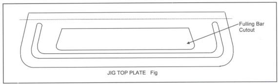
For the jig with fullness, the template should be prepared with a fullness cut out for the stylus to follow, see figure 1.3. The shape of this cut out is determined by the setting of oddleg scribers to the width required between the fulling bar and edge of template. Scribe round the edges of the template and draw a line parallel to the hinge line to give required width of fulling bar. Make an allowance for difference between cutter and stylus.
